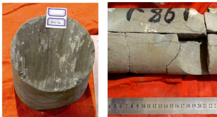
Figure 1 Xingshugang oilfield Fuyu Reservoir fracture characteristics
